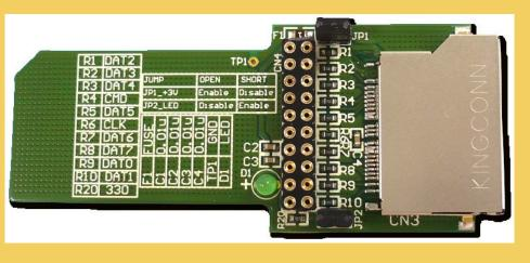
The SD Extender 1.0 is a debug and signal detection tool for Secure Digital Memory Card. It allows a Secure Digital Memory Card to be extended from the host slot for full access to the all of signal pins.
