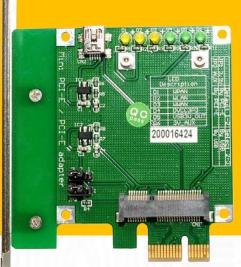
The PCI-E Mini Card adapter is designed for desktop PCs that converts PCI Express Mini Card to USB and standard PCI-Express 1x slot.
