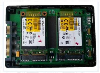
B: Connect SATA 15pin powered SSDMR directly to the computer. Work in FAST mode Device manager
