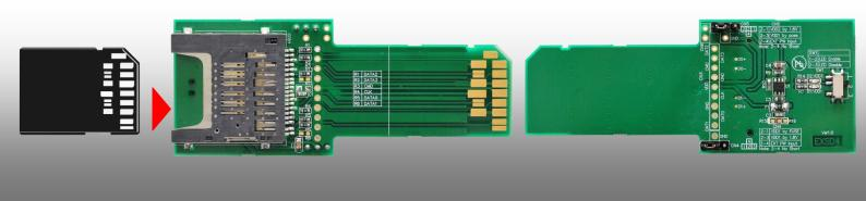
The **EXSD4** is a debug and signal detection tool for Micro Secure Digital Memory Card. It allows a SD 4.0 card to be extend from the host slot for full access to the all of signal pins. UHS-II mode with maximum 312MB/s speed and UHS-I mode with maximum 104MB/s are supported. It also allows application of other Secure Digital Memory Card on the equipment which has SD card interface.
